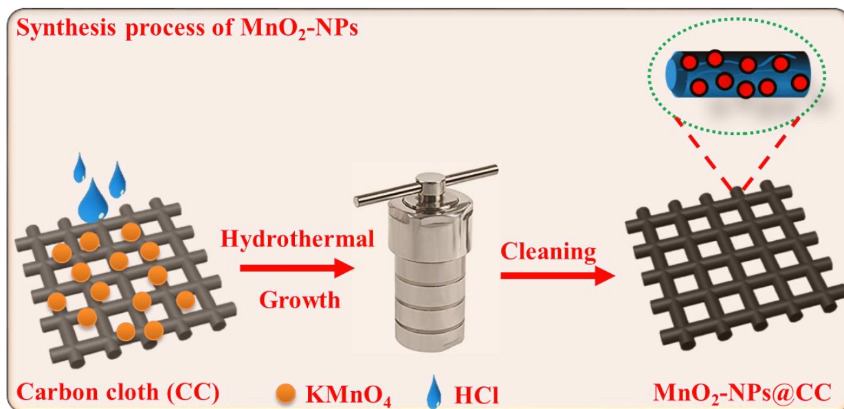
Figure 1. Schematic representation of a typical synthesis procedure of MnO 2 -NPs@CC.
