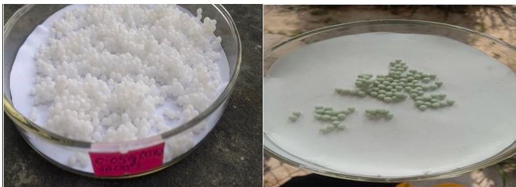
Fig. 2. High resolution optical images of 3NMC-MCA-TiO 2 hydrogel composite beads: (a) before Cu(II) sorption, (b) After Cu(II) sorption.
