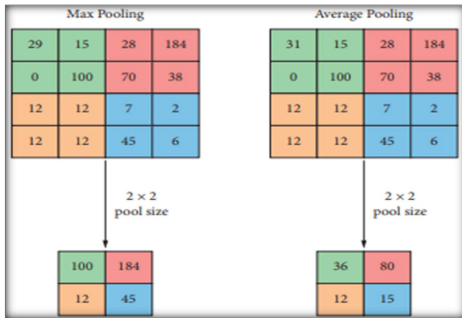
Fig. 10 Pooling function of CNN model
